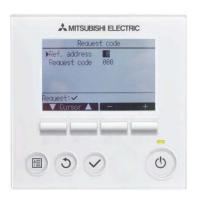
5. In the Request code screen enter the outdoor unit address and the appropriate rotation setting - see list on reverse.
