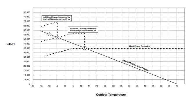
(L) Calculated heat loss at outdoor design temperature
